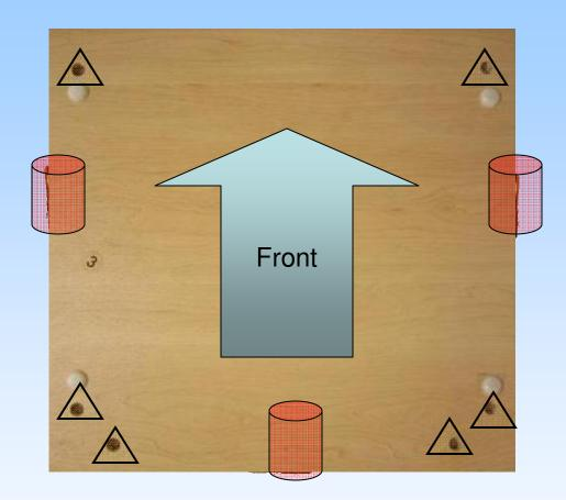
Insert six # B screw caps highlighted with  $\bigwedge$  on outside of # 3 bottom panel (shorter) Flip over the bottom panel and attach three corner braces highlighted with to inside of # 3 panel using # E screws
