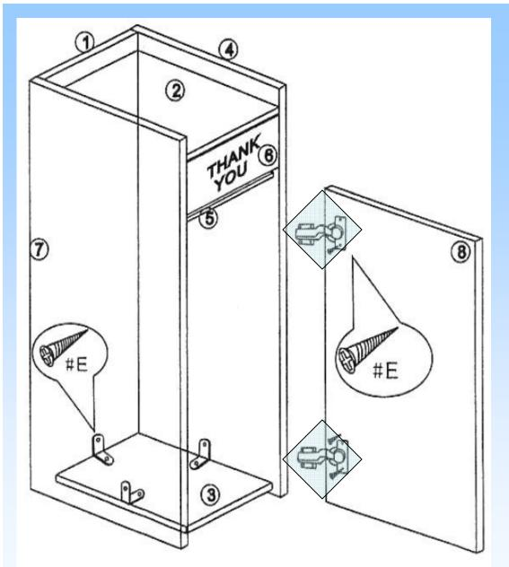
Screw in the hinges highlighted with to # 8 door then attach # 8 door to # 4 panel with four # E screws
