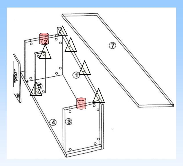
Flip over panel set assembled in previous step; attach # 6 and # 5 panel to # 4 panel; attach # 7 as shown; then tightening all # B screw cap highlighted with  $\triangle$  180 degree clockwise to lock.
