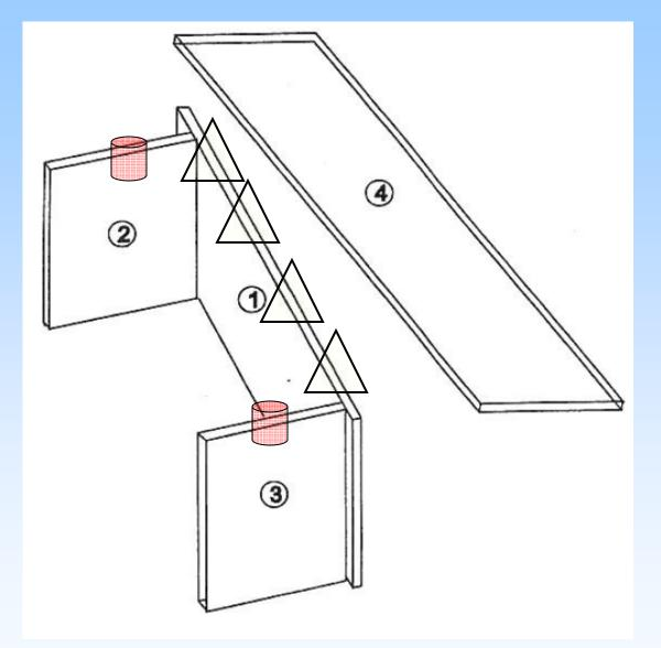
Attach #4 panel to the right of the panel set assembled in previous step; tightening # B screw cap highlighted with 180 degree clockwise to lock
