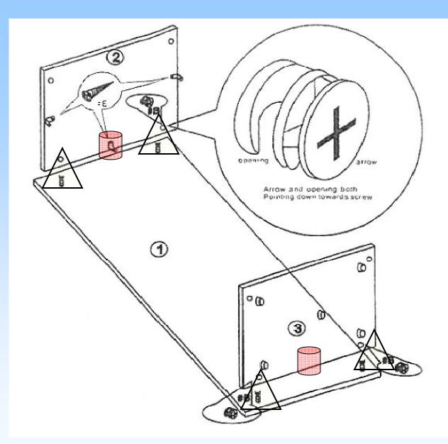
Attach #2 and #3 panels to # 1 panel by tightening # B screw cap highlighted with 180 degree clockwise to lock Secure corner braces Highlighted with by using # E screws
