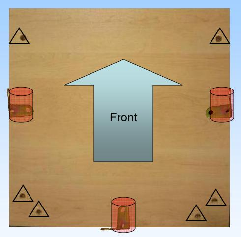
Insert six # B screws highlighted with \_\_\_\_\_ on # 2 top panel (longer)
