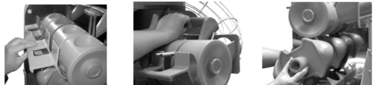
Remove the squeezer drum by unscrewing the screw. Remove the second squeezer male part.
