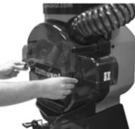
Remove the front cover, by unscrewing the two lateral screws.
