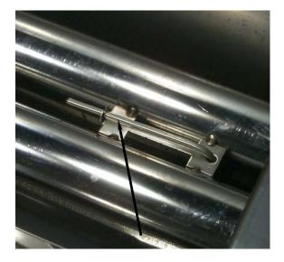
Electronic thermostat probe in frypot (arrow).
