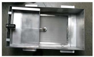
Crumb screen properly placed in filter pan.
