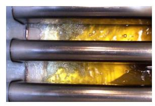
Polishing the oil removes suspended particles, which increases the life of the oil.
