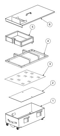
A filter unit which utilizes disposable filter paper to filter oil.
