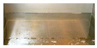
Add oil/shortening until the oil level is at the top OIL LEVEL line. DO NOT OVERFILL THE FRYPOT.
