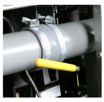
Pull the yellow handle to open the oil return valve and activate the filter pump.
