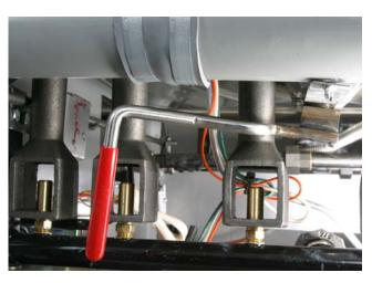
After filtering is complete, close the red drain handle to start refilling the frypot.
