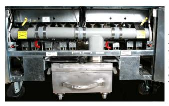
The filter pan slides under the fryer (left), connecting with a male connector (right). Ensure that the pickup tube is securely coupled with this connector. Its location may vary based on model.
