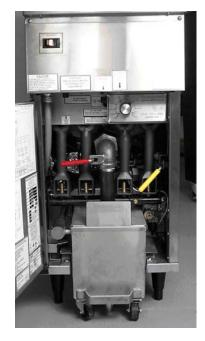
Typical Single Under Fryer Filter (SUFF) installed in a single fryer.
