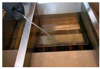
Removing support grid from fry vessel prior to filtering.
