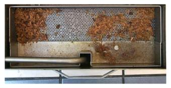
Empty the filter pan crumb tray into a fire-proof container at the end of frying operations each day. DO NOT ALLOW CRUMBS TO ACCUMULATE IN TRAY.
