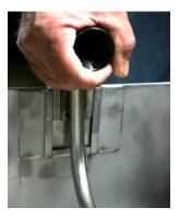
Carefully remove the filter leaf assembly.
