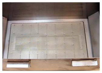
Support grid properly placed in filter pan.
