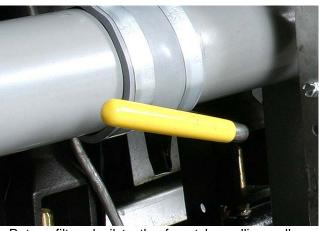
Return filtered oil to the frypot by pulling yellow handle to open oil return valve.
