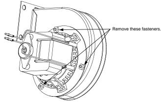
3. Wrap the motor with plastic wrap to prevent water from entering it. Spray degreaser or detergent on the blower wheel and the blower housing. Allow it to soak for five minutes. Rinse the wheel and housing with hot tap water, then dry with a clean cloth.
