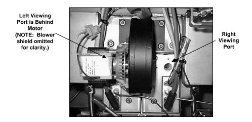
The air/gas mixture is properly adjusted when the burner manifold pressure is in accordance with the applicable table on page 2-7 and the burners display a bright orange-red glow. If a blue flame is observed, or if there are dark spots on a burner face, the air/gas mixture requires adjustment.
