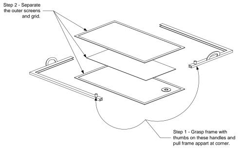
2. Separate the outer screens and grid.
