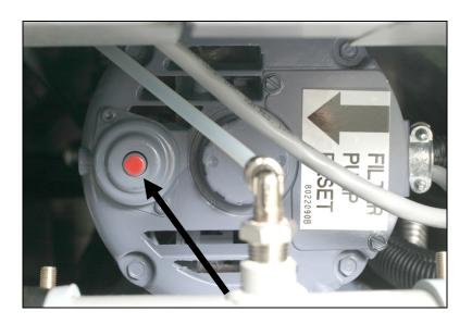
**Filter Pump Reset Switch**
