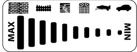
**NOTE:** To apply chemicals the black low pressure nozzle must be installed and the Dial-N-Wash must be in the MAX pressure setting.
