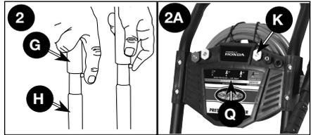
4. Remove the colored quick-connect nozzles (K) from the plastic bag and insert them into correct grommet on the nozzle holder. Nozzles are color coded to match colored nozzles on label (Q).
