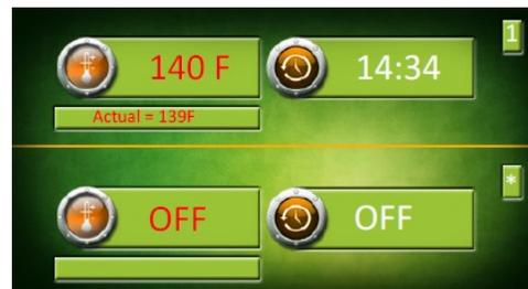
Step 5: Program the “Bottom Zone” by pressing one of the bottom OFF buttons on the main menu screen
