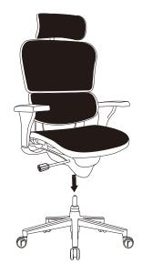
Now turn the assembled seat upright and locate the center hole of the Mechanism over the Seat Post. Push down firmly until the connection is secure.
