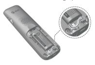
2. Align the cover flat against the battery compartment, then slide it upwards until it clicks into place.
