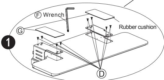
Connect and fix the junction plate and keyboard tray by 8 screws and use the wrench F to fasten afterwards.
