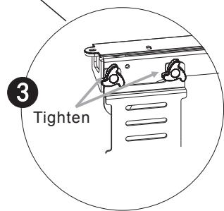
Hang the junction plate on the knob assembly and then tighten the knobs.
