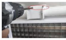
6. Remove the 2 screws which are securing the water pump.
