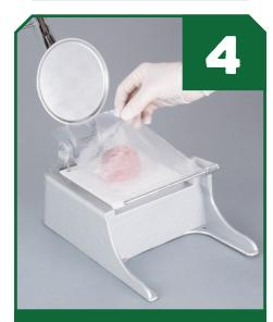
Ensure the loop of the plastic liner is attached to the metal rod on the base. Place the liner on top of the ground meat.
