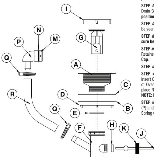
**STEP #1:** Remove locknut (D), Rubber Gasket (C) and cardboard Gasket (B) from Drain Body (A). Slip drain body into 3 1/2" sink opening. Place sealing compound between flange of drain body and sink. With the Drain Body (A) protruding from the bottom of the sink, place the Rubber Gasket (C), then Cardboard Gasket (B) over Drain Body and secure in place with Locknut (D).
