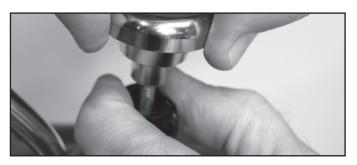
Pull down on grooved sleeve until it separates from knob. Turn knob counter clockwise for a larger portion and clockwise for a smaller portion. Release sleeve and turn knob slowly until the pins on top of sleeve seat into the holes on underside of knob. Test the pump with the condiment to be dispensed and make additional adjustments if necessary.
