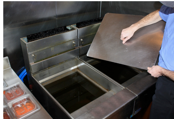
Step 1-Cover equipment before cleaning.
