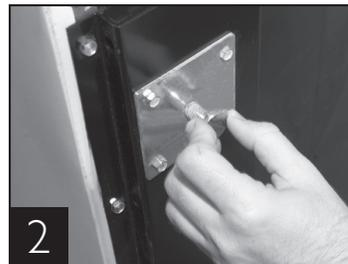
2 Reinstall leg levelers at bottom of cabinet.
