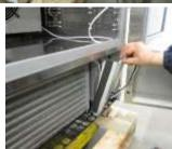
Remove the electrical panel locking screw.
