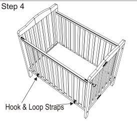
Unfasten the two hook & loop straps from the rail (A) and drop posture board down into position. Fasten the posture board with hook &loop straps to side rail (B)
