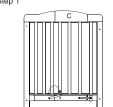
Before assembly drop the two latches on the end panels (C).
