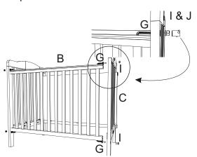
Insert swivel pins (G) into the remaining side rail (B) as illustrated. Insert the threaded end of swivel pin into end panel (C). Tighten with nuts (I) using wrench (J).
