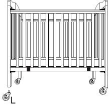
Insert the four castors (L) into the leg posts
