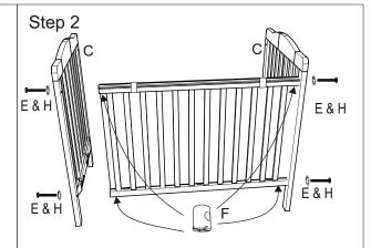
Insert 4 barrel nuts (F) under the horizontal posts. Attach one end panel (C) to rail (A) using four bolts (E) & lock washers (H). Tighten with allen wrench (M). Repeat step with remaining end panel (C) Note: Latches at bottom of end panel are inside the crib.
