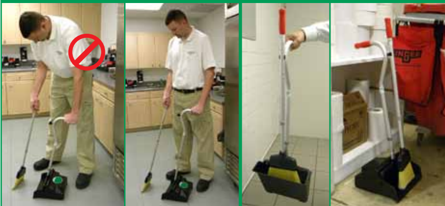
A longer, adjustable handle on both tools eliminates bending - which produces strain.
