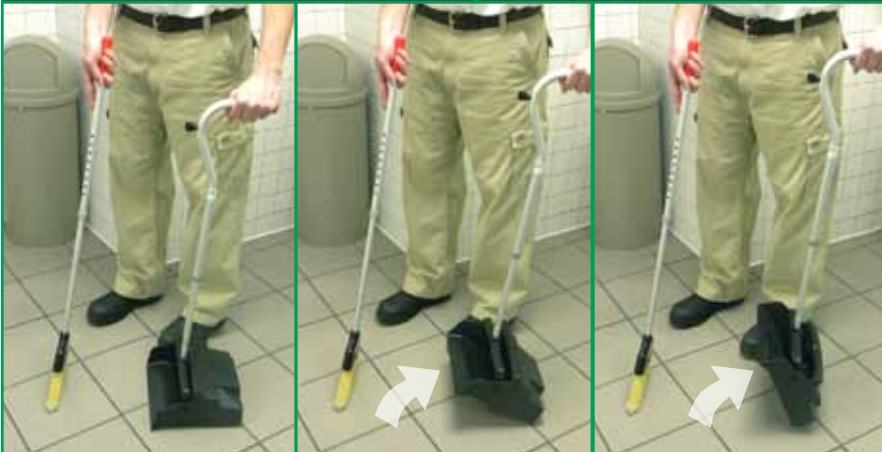
The telescopic dustpan retracts upwards when lifted. This eliminates the possibility of debris falling from the dustpan while being moved from area to area.
