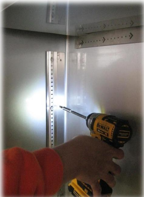
Remove the pilaster strips from the sides of the cabinet. Then install the side pilaster support brackets in these holes. (Leave the bottom screw out until the Bottom Rear Bracket is installed.)
