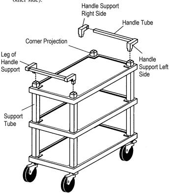
**NOTE:** The direction of the leg of the handle support is pointing away from the cart.
